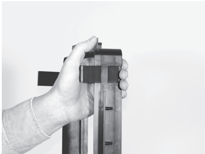
Fig. 2 Installing the clamping tabs
